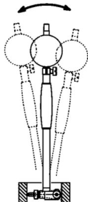
position of the bore gauge must be the same as in the measurement.
