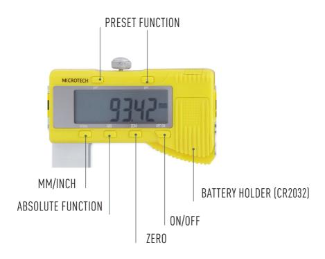
For activating PRESET function press ZERO button during 5 sec (only in ABS mode) SET indication will be on screen durring PRESET activated. With buttons PRE + and PRE - possible set preset value.
